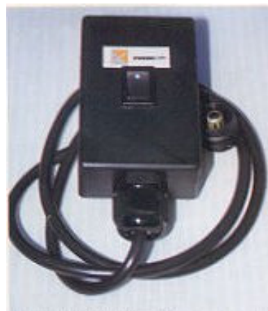
PLUG-IN TECHNOLOGY, like this unit which accesses the Mercedes Benz ECU via the diagnostic port, has opened up a vast new potential for cars thought to be 'unchippable'.
